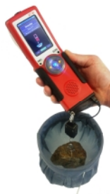
Density Measurement: Sample Submerged in Water
