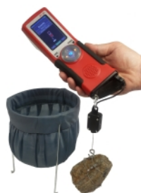
Density Measurement: Sample in Air
