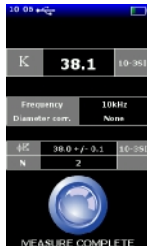
Discrete Magnetic Susceptibility Measurement
