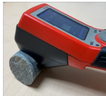
Curved Sensor Measuring Core Sample
