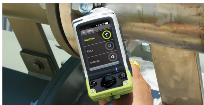
The Niton XL5 Plus in use, analyzing a tight weld in an oil refinery.
